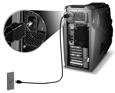
2 Plug the other end of the power cable into a power outlet.
