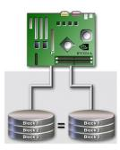
RAID 5 : Defines techniques for parity data. Data is striped and parity is distributed across three or more drives, improving disk performance and fault tolerance.
