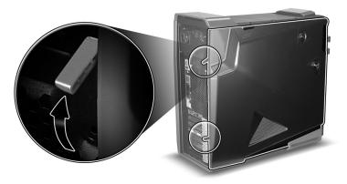
(2) Hold the rear edge of the panel with both hands then slide the panel towards the rear of the chassis.
