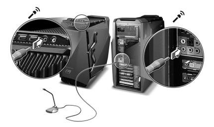
Amplified stereo speakers, headset, or heaphone — Plug amplified speakers, headset, or headphone to the headphone/line-out/front speaker jack (green jack) located on the front and rear of the computer.
