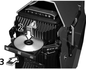
3. Push the tray and it will close automatically or press the eject/load button.
