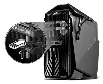
When the disk tray slides open, place the disk gently on the tray. Make sure that the label or title side of the disk is facing upward.
