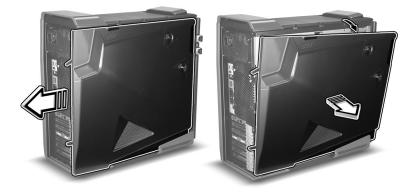
(3) Lift the panel upward to detach it.
