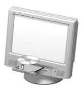
4. Gently press the CD down to make sure that it is properly inserted.
