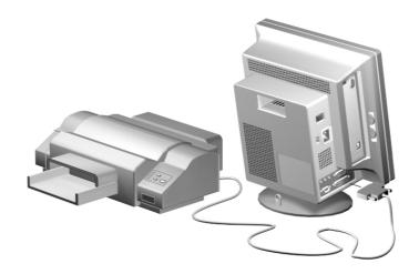
To connect a serial printer, plug the printer cable into the serial port [IDIO] (teal or turquoise port) located on the left panel of your computer. See "Left panel" on page 13 for the location of the serial port.
