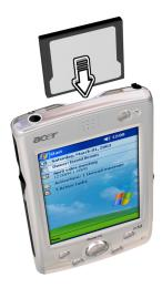
4 Push the card into the slot using your finger until you feel the card lock and hear an audible system sound; this will signal that the card is already properly seated within the slot.
