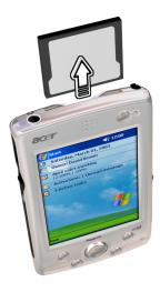
When your handheld emts a two-tone beep you have properly removed the card. Reinsert the dummy CF card to protect the connectors.
