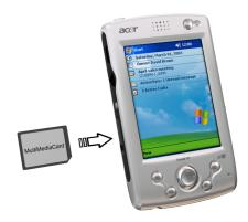
Push the card into the slot using your finger until you feel the card lock and hear an audible system sound. This indicates that the card is properly seated within the slot.
