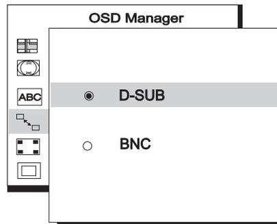
There are two kinds of input connectors for Acer 211c. One is a BNC connector, the other is a DB-15. The Acer 211c is capable of automatically detecting the type of connector used (either BNC or DB-15). If the two connectors are connected simultaneously, the user can select the desired connector.
