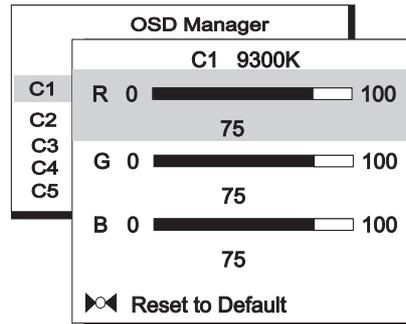
This sub-menu adjusts RGB (Red, Green, Blue) color weight. Press ▲ or ▼ keys to scroll light coloured bar to desired items then press ◀ or ▶ key to do the adjustments.
