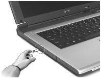
When the power is off, you can eject the drive tray by using the emergency eject hole.
