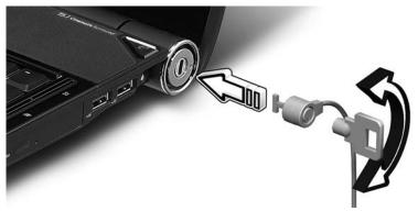
Wrap the computer security lock cable around an immovable object such as a table or handle of a locked drawer. Insert the lock into the notch and turn the key to secure the lock. Some keyless models are also available.
