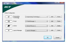
Launch Manager allows you to set the easy-launch button located above the keyboard. **"Easy-launch buttons" on page 26** for the location of the easy-launch buttons.
