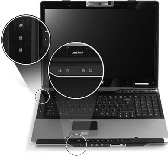
The power, battery and wireless communication status indicators are visible even when the LCD display is closed.
