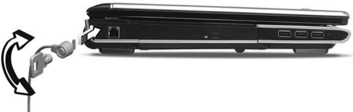
Wrap the computer security lock cable around an immovable object such as a table or handle of a locked drawer. Insert the lock into the notch and turn the key to secure the lock. Some keyless models are also available.
