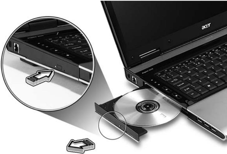
Insert a clip to the emergency eject hole to eject the optical drive tray when the computer is off.
