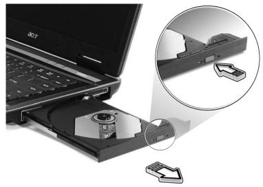
Insert a paper clip to the emergency eject hole to eject the optical drive tray when the computer is off.
