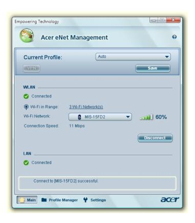
Acer eNet Management can save network settings for a location to a profile, and automatically switch to the appropriate profile when you move from one location to another. Settings stored include network connection settings (IP and DNS settings, wireless AP details, etc.), as well as default printer settings. Security and safety concerns mean that Acer eNet Management does not store username and password information.
