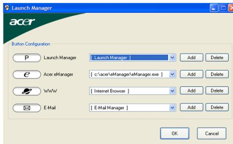
Launch Manager allows you to set the four easy-launch buttons located above the keyboard. See **"Easy-launch buttons"** on page 10 for the location of the easy-launch buttons.
