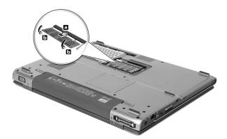
4 Replace the memory cover and secure it with the screw.
