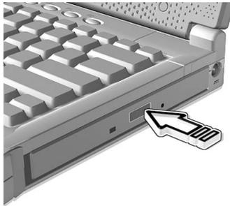
When the power is off, you can eject the drive tray using the emergency eject hole. See page 46.
