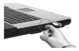
When the power is off, you can eject the drive tray using the emergency eject hole. See page 46.
