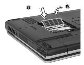
4 Replace the memory cover and secure it with the screw.
