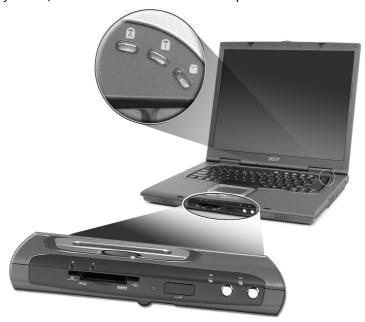
The Power and Battery status indicators are visible even when the display is closed.
