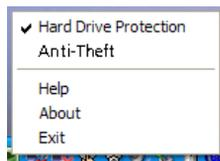
Selecting this function will park the HDD heads in the event that any vibration or movement which exceeds the level tolerated by the HDD is detected.
