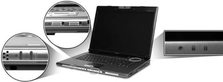
The power, battery, Bluetooth and wireless communication status indicators are visible even when the LCD display is closed.
