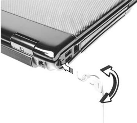
Wrap the computer security lock cable around an immovable object such as a table or handle of a locked drawer. Insert the lock into the notch and turn the key to secure the lock. Some keyless models are also available.
