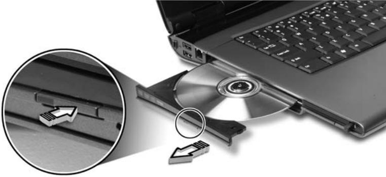
Insert a clip to the emergency eject hole to eject the optical drive tray when the computer is off.
