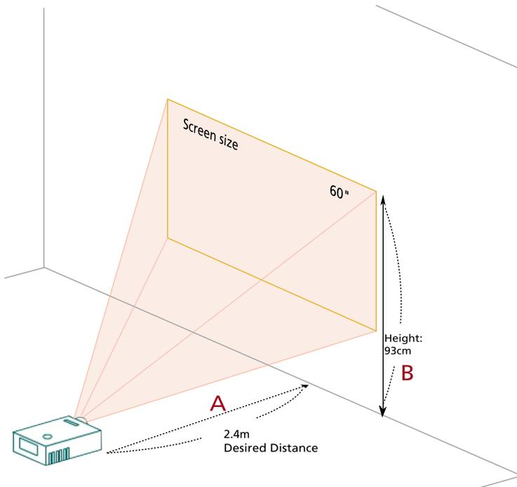
**Figure:** Fixed distance with optimal screen size.
