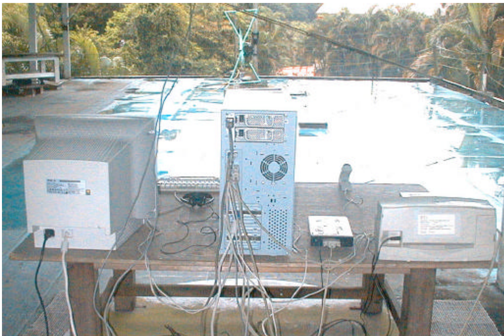
Back View of Highest Radiated Emission Test.
