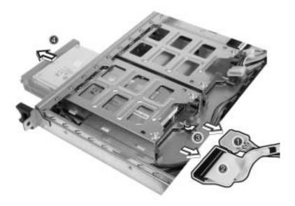
4 Remove the screws that secure the hard disc to the disc tray (1) and remove the drive from the tray (2). Keep the screws for later use.
