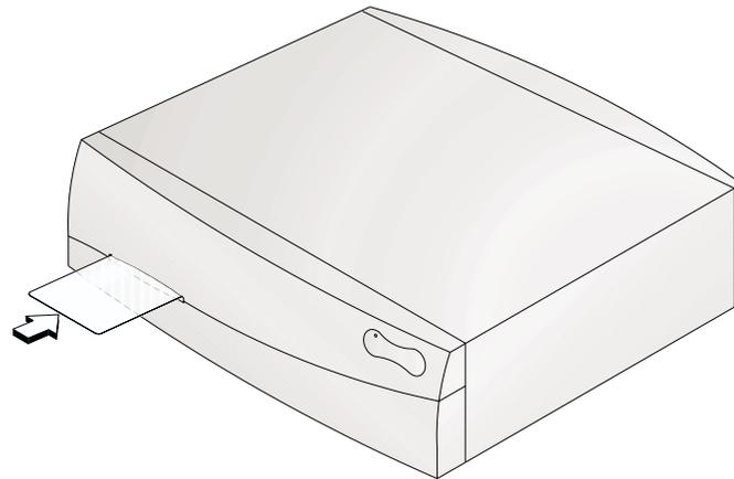
3. After inserting the SmartCard, the system will boot up and the Acer logon screen will be displayed.
