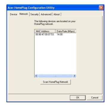
**Network**– This tab will show all HomePlug devices connected to the network. Scan the network for newly added devices.
