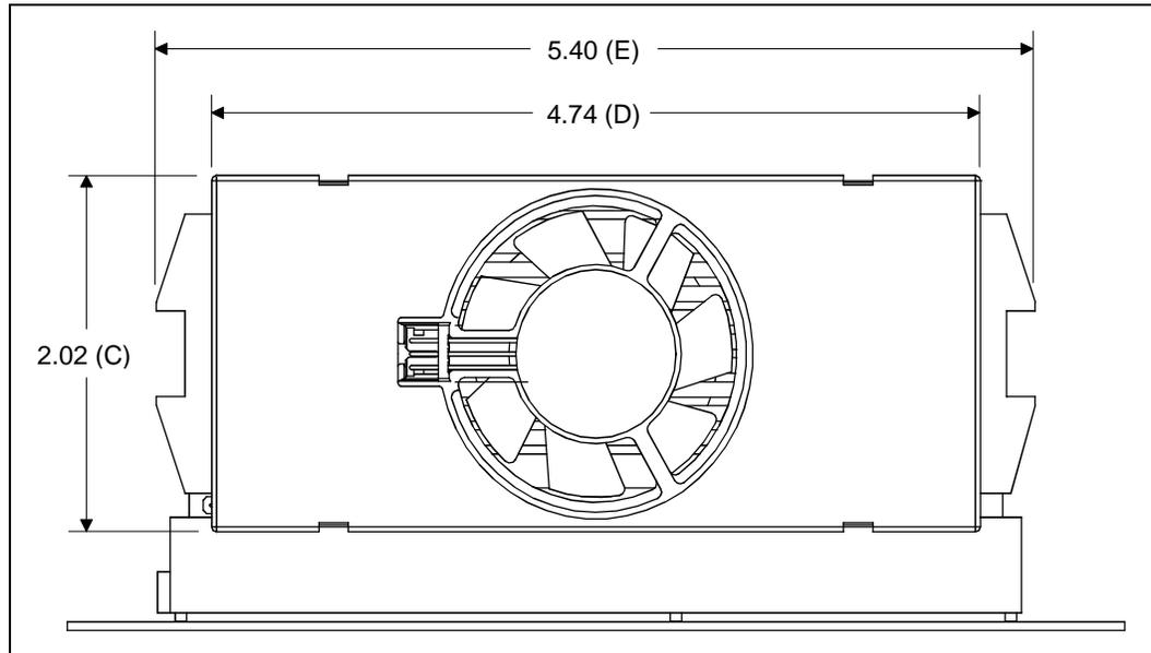
Figure 21. Top View Airspace Requirements for the Boxed Processor
