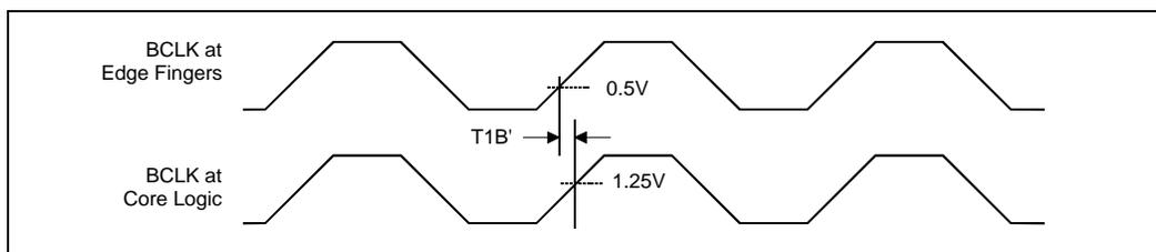
**Figure 3. BCLK\*, PICCLK, and TCK Generic Clock Waveform**
