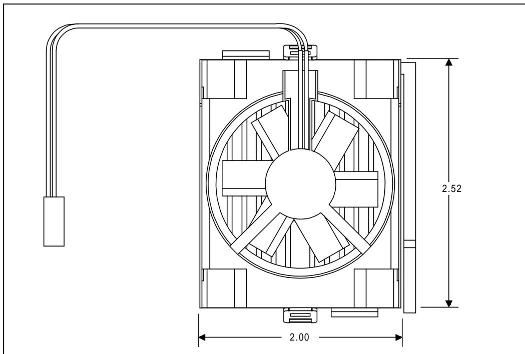
**Figure 27. Side View Airspace Requirements for the Boxed Processor**
