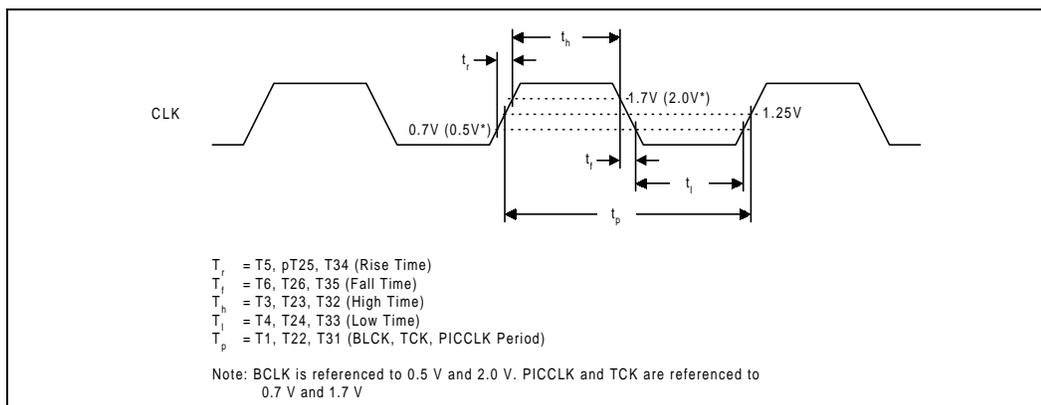
Figure 4. Intel® Celeron™ Processor System Bus Valid Delay Timings
