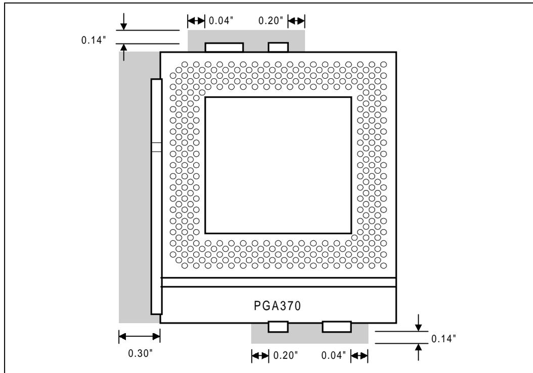
Figure 31. Side View of Motherboard Keepout Requirements
