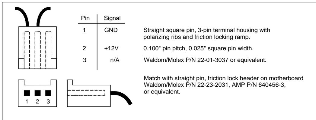
Table 41. Fan Heatsink Power and Signal Specifications
