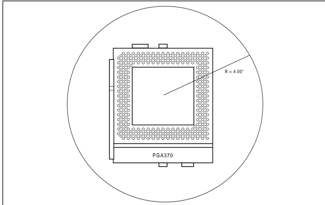
Figure 30. Top View of Motherboard Keepout Requirements
