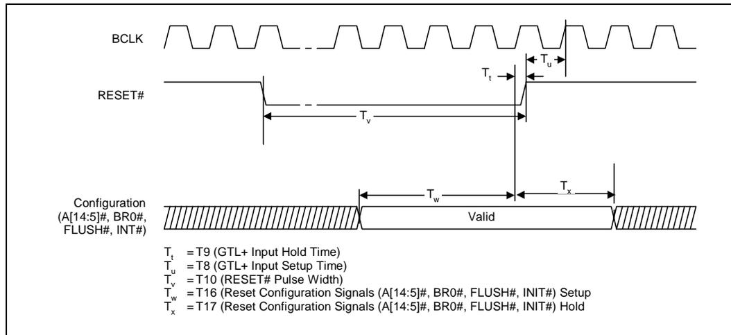
Figure 7. Power-On Reset and Configuration Timings
