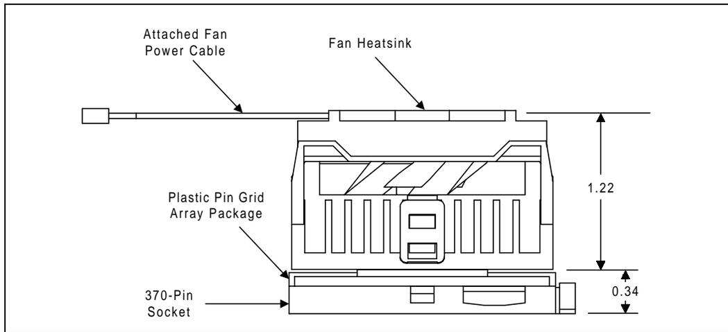
Figure 26. Top View Space Requirements for the Boxed Processor
