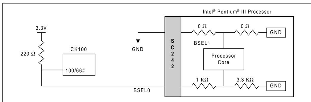
**Figure 5. BSEL[1:0] Example for a 100/133 MHz Capable System (100 MHz Processor Installed)**
