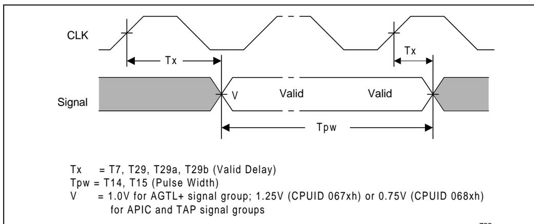
Figure 9. System Bus Setup and Hold Timings
