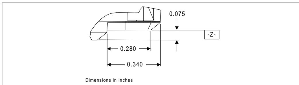
Figure 37. S.E.C.C.2 Packaged Processor Substrate — Edge Finger Contact Dimensions
