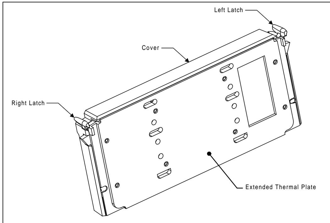
Figure 19. S.E.C.Cartridge 2 — Substrate View
