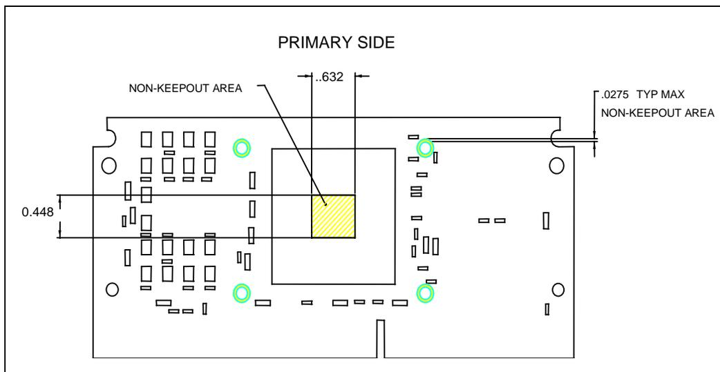
Figure 41. S.E.C.C.2 Packaged Processor Substrate (CPUID 067xh) — Keep-Out Zone
