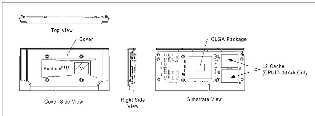
Figure 32. S.E.C.C.2 Packaged Processor Assembly — Primary View
