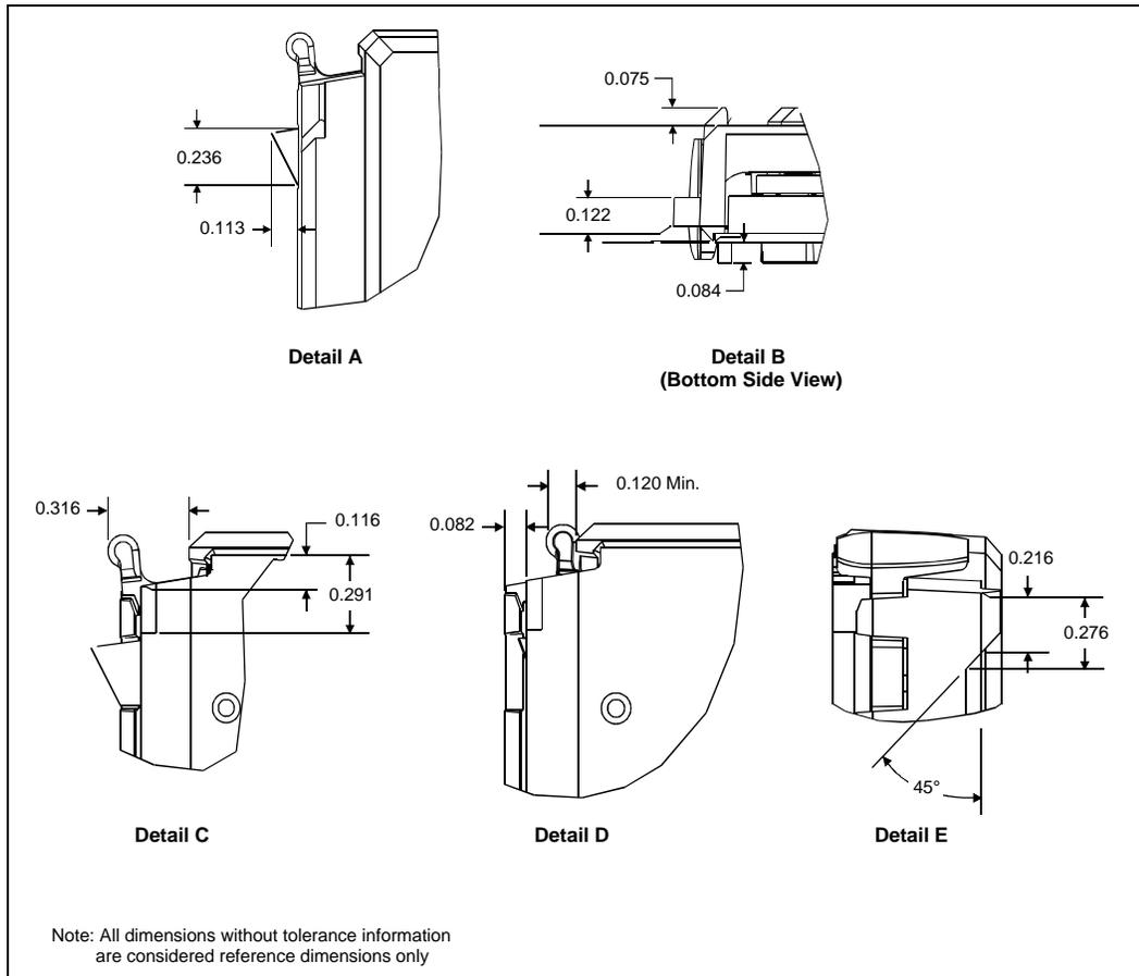
Figure 26. S.E.C.C. Packaged Processor — Extended Thermal Plate Attachment Detail Dimensions
