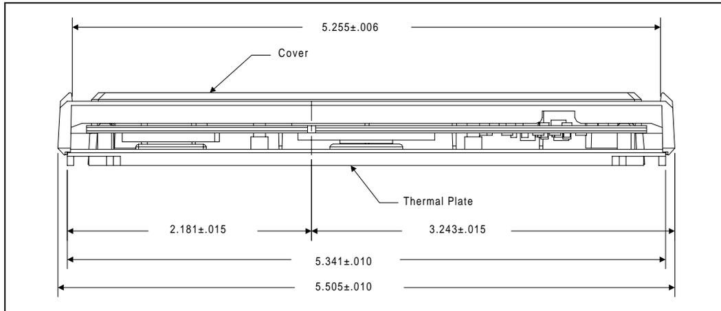
Figure 24. S.E.C.C. Packaged Processor — Latch Arm, Extended Thermal Plate Lug, and Cover Lug Dimensions
