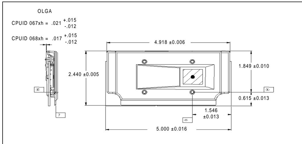
Figure 34. S.E.C.C.2 Packaged Processor Assembly — Heat Sink Attach Boss Section
