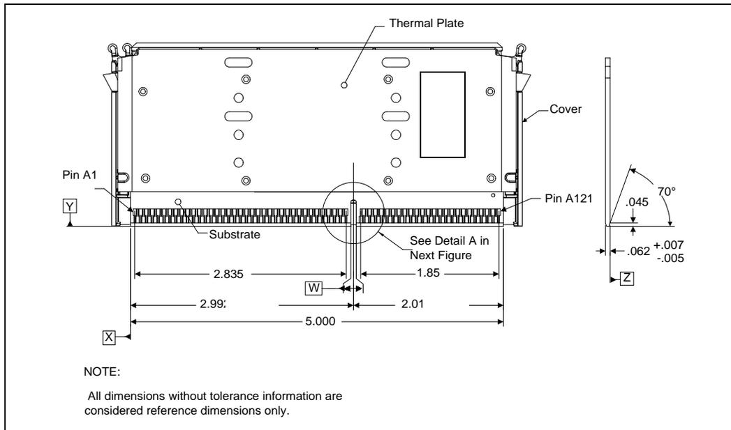
Figure 29. S.E.C.C. Packaged Processor Substrate — Edge Finger Contact Dimensions, Detail A
