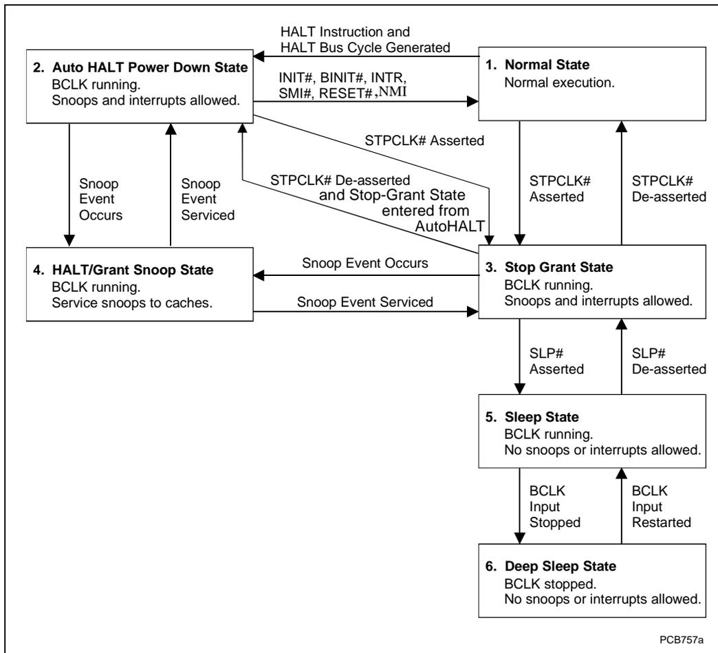
For the processor to fully realize the low current consumption of the Stop-Grant, Sleep, and Deep Sleep states, a Model Specific Register (MSR) bit must be set. For the MSR at 02Ah (Hex), bit 26 must be set to a '1' (this is the power on default setting) for the processor to stop all internal clocks during these modes. For more information, see the *Intel Architecture Software Developer's Manual, Volume 3: System Programming Guide* (Order Number 243192).
