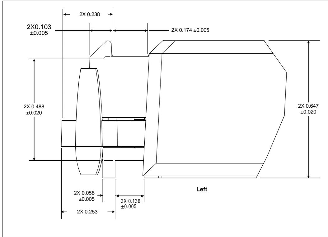
**Figure 25. S.E.C.C. Packaged Processor — Latch Arm, Extended Thermal Plate, and Cover Detail Dimensions (Reference Dimensions Only)**
