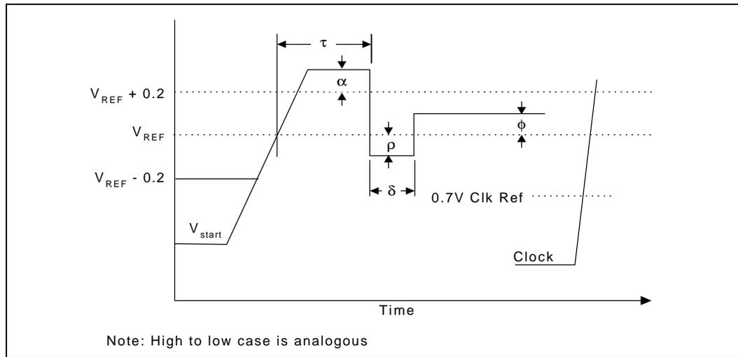
Figure 17. Signal Overshoot/Undershoot, Settling Limit, and Ringback <sup>1</sup>
