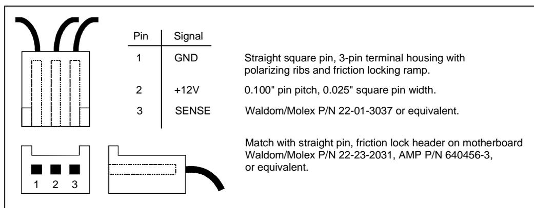
Table 39. Fan Heatsink Power and Signal Specifications
