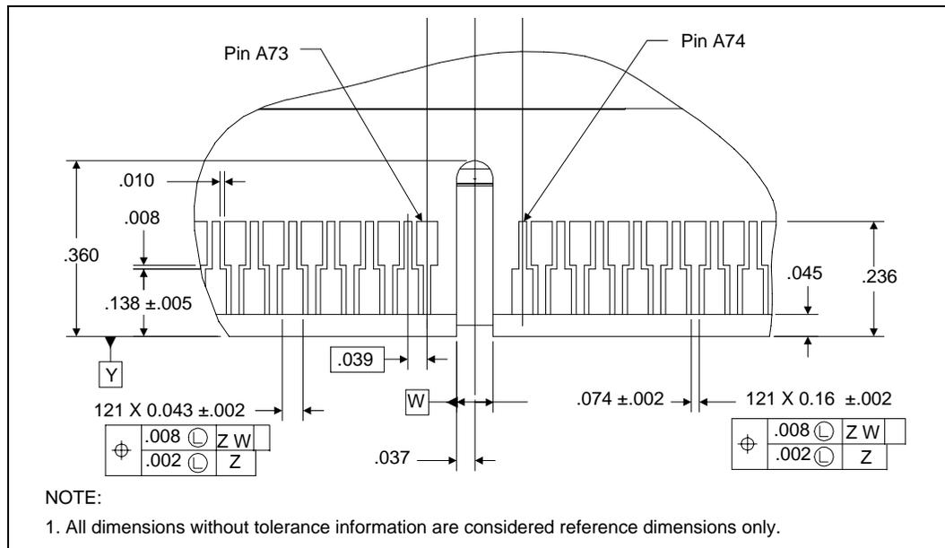
Figure 39. S.E.C.C.2 Packaged Processor Substrate (CPUID 067xh) — Keep In Zones
