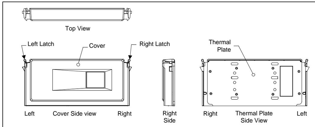
Figure 22. S.E.C.C. Packaged Processor — Extended Thermal Plate Side Dimensions
