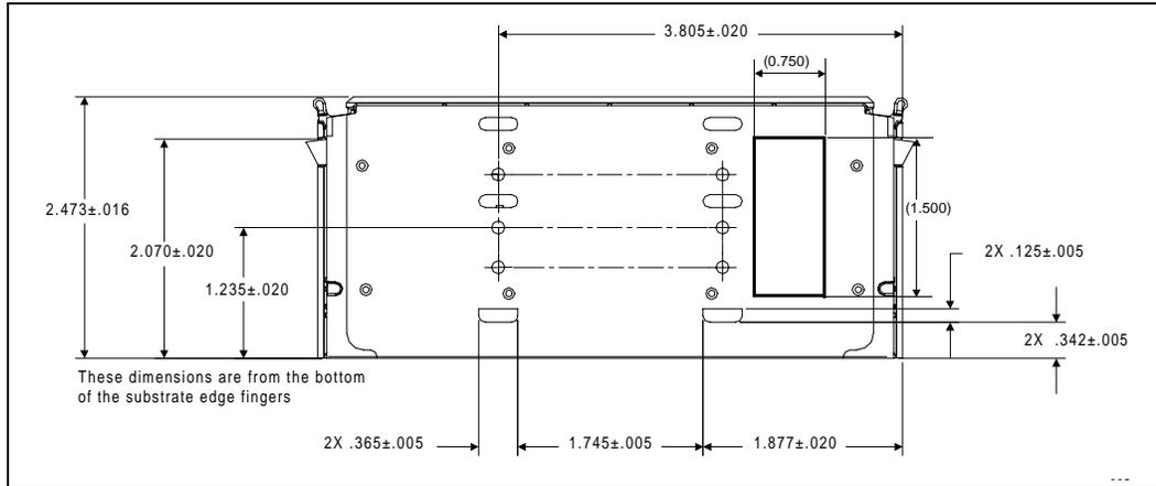
Figure 23. S.E.C.C. Packaged Processor — Bottom View Dimensions
