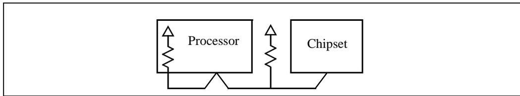
Figure 3. AGTL+ Bus Topology in a Dual-Processor Configuration
