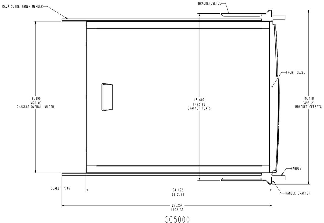
Figure 6: SC5000 Chassis and AHDRACK kit dimensions
