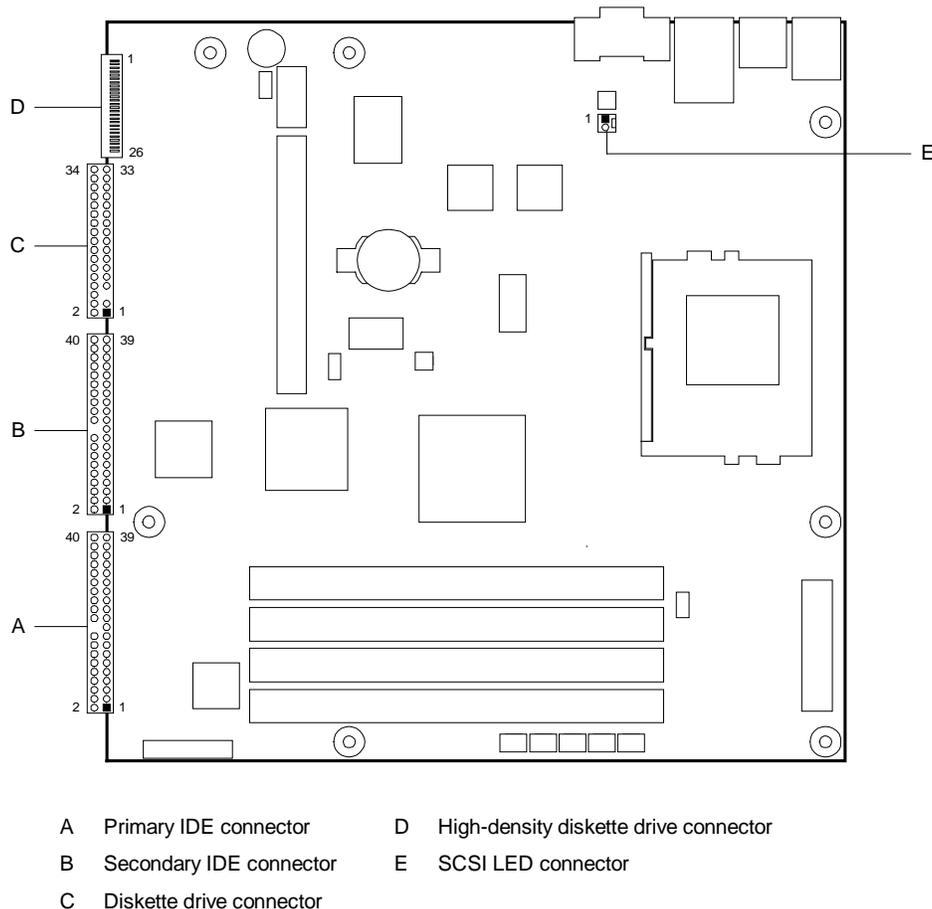
**Figure 11: Peripheral connectors**
