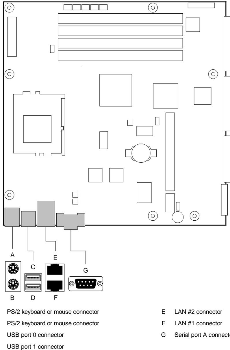
**Figure 10: Back panel I/O connectors**
