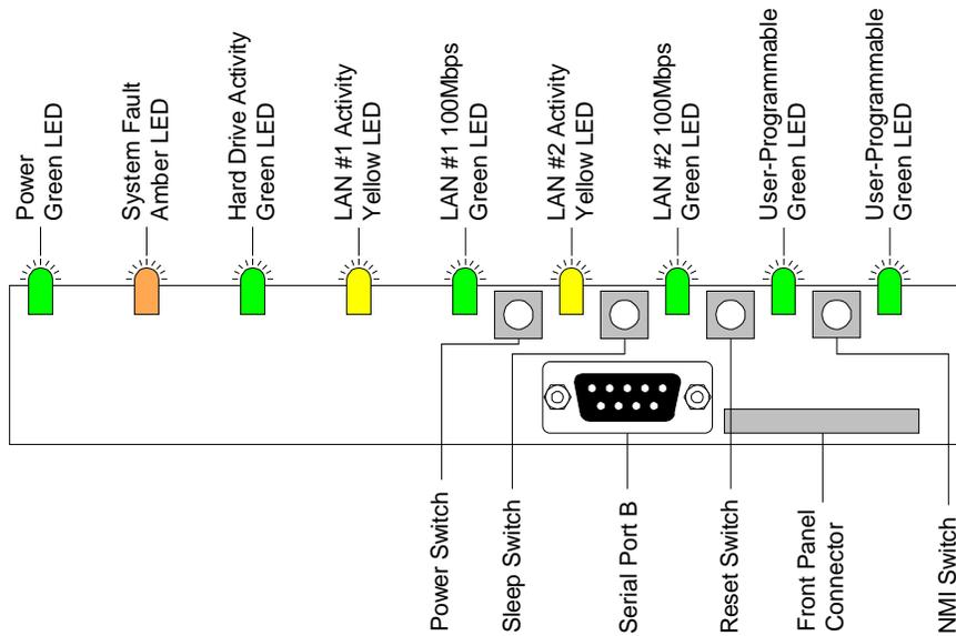
**Figure 19: Front panel board**
