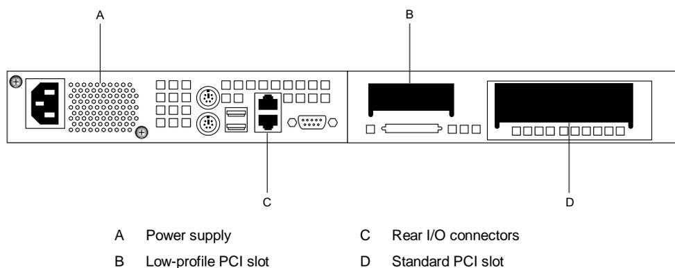
**Figure 3: Rear view of chassis**
