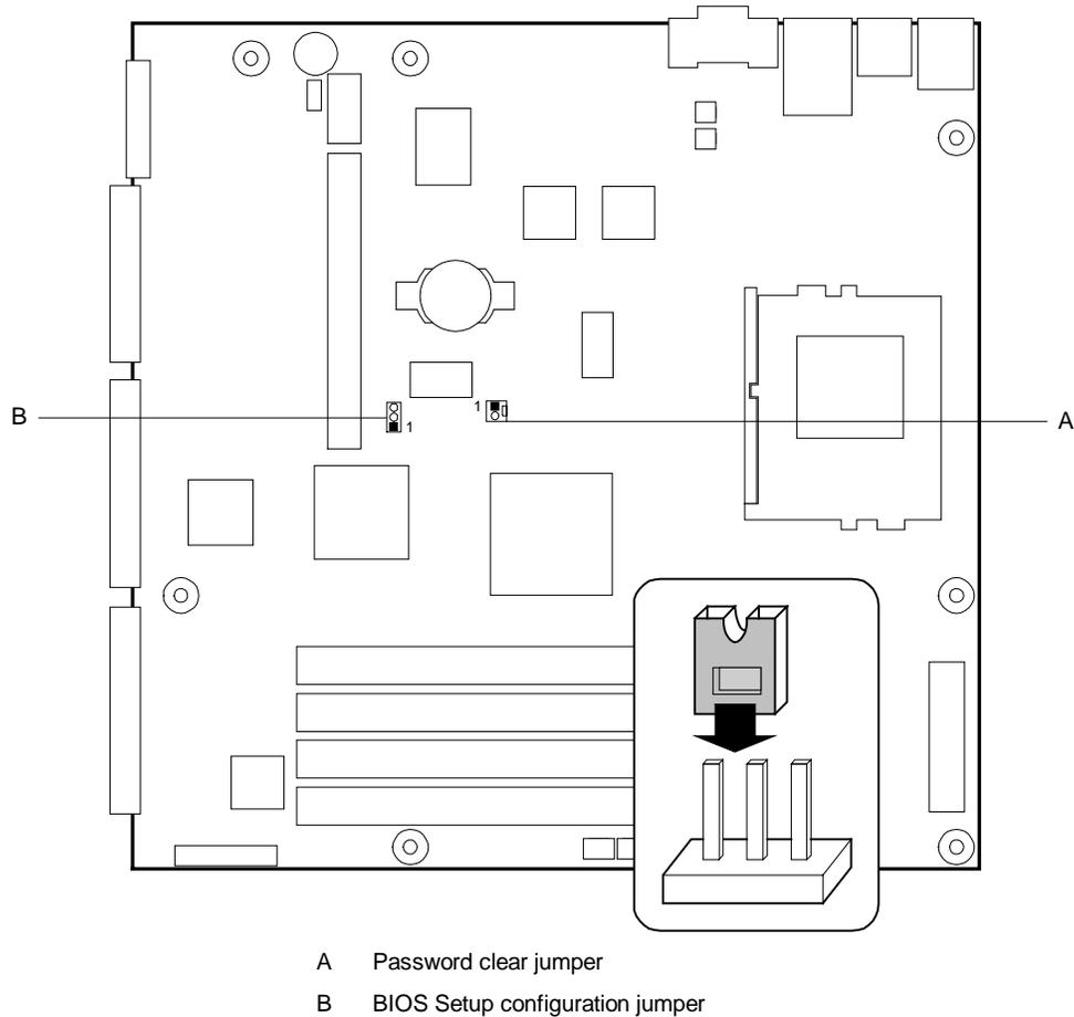
**Figure 15: BIOS Setup configuration and password override jumpers**
