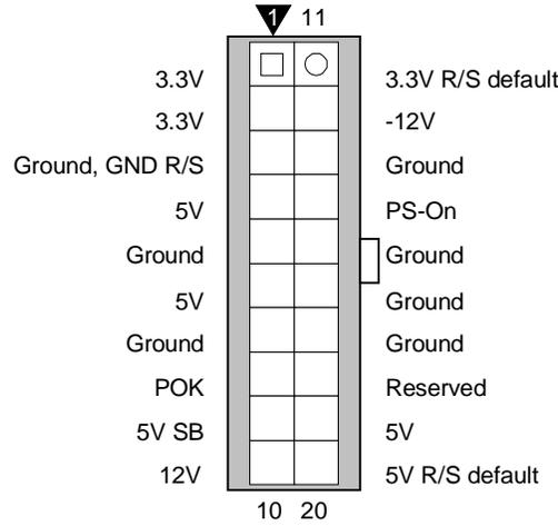
Figure 4: DC connector pinout
