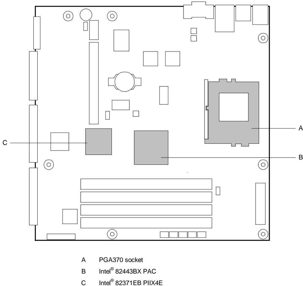
**Figure 17: Thermally-sensitive components**
