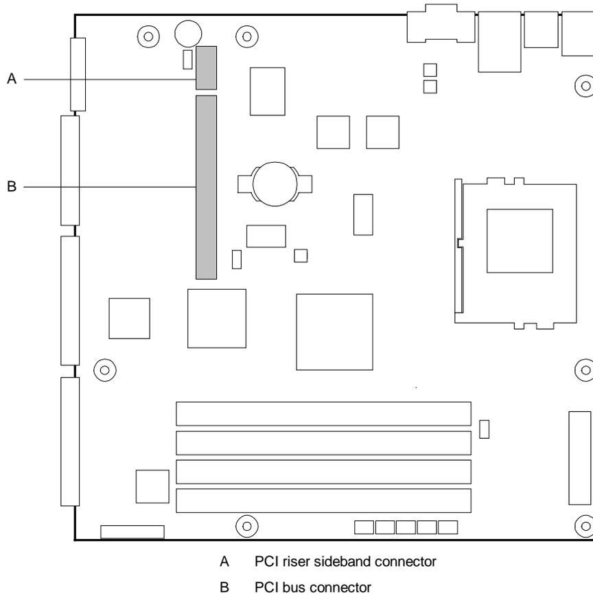
**Figure 13: PCI riser sideband and PCI bus connectors**
