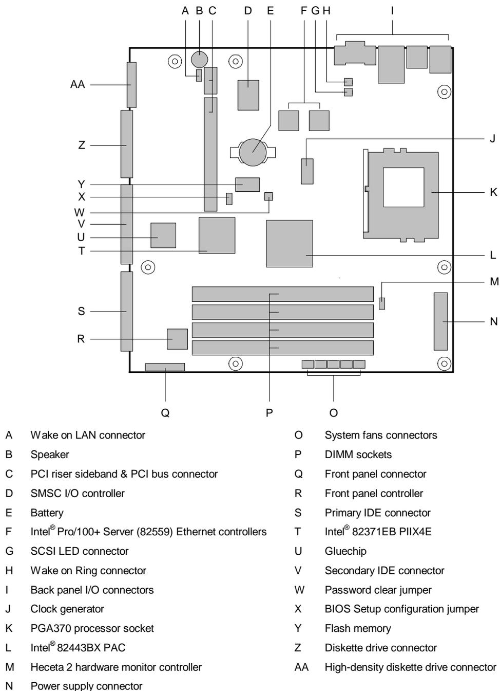
**Figure 7: Serverboard components**
