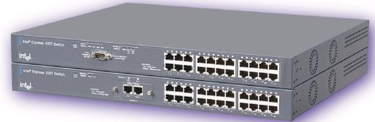
switch to meet additional aggregated bandwidth. By stacking these Layer 2 switches, you can deliver more dedicated user bandwidth to expanding workgroups as you need it, while controlling network costs. The Intel® Express 530T Switch provides switching control for the Intel® Express 535T Switch. Stack up to four switches for a total of 94 auto-negotiating ports of non-blocking performance.
