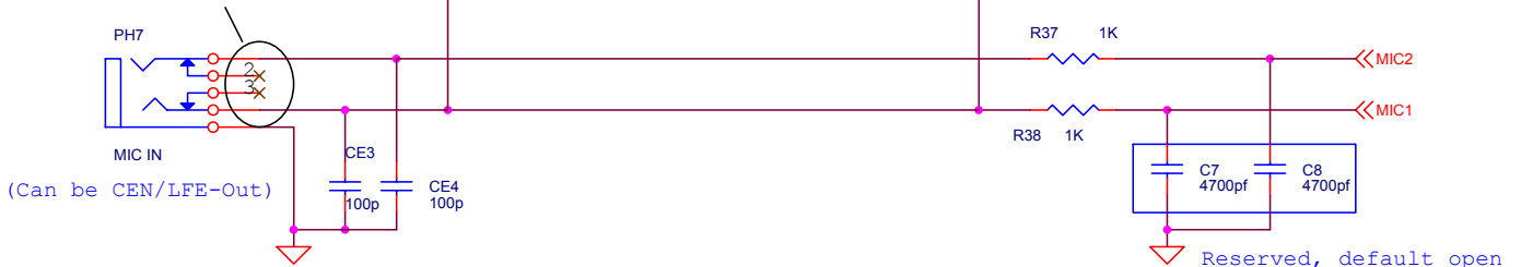
Analog I/O connection of the ALC650
