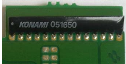
Figure 1. Konami resistor ladder soldered into the SCC-based cartridge
