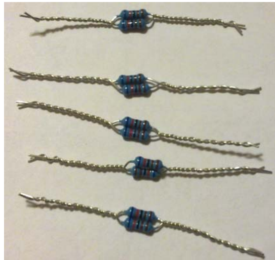
(d) connect 8 pairs of the resistors to form a circuit of twice less nominal
