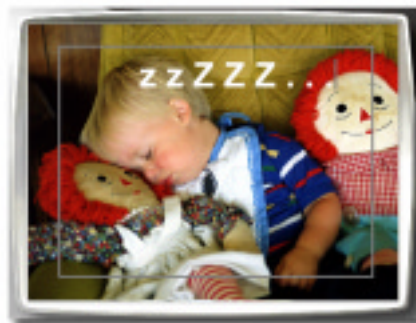
A centered title being edited. Note the Title safe area around the center of the window.
