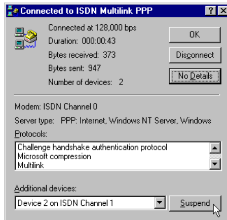
FIGURE 2-13: DIAL-UP NETWORKING CONNECTION STATUS
