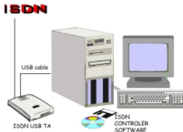
FIGURE 1-1: THE ISDN SYSTEM
