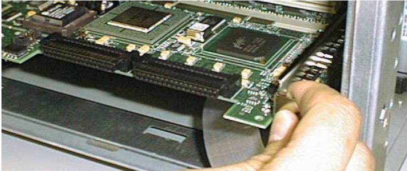
Figure 5. Plugging the AcceleRAID 352 into a PCI Slot
