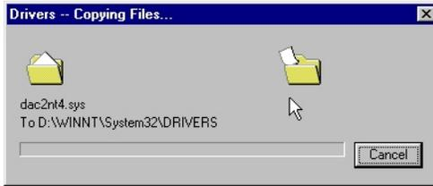
**Figure 3-9. Install the New Driver from Diskette**
