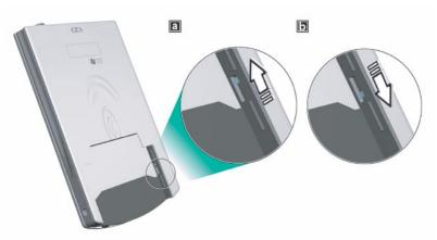
3 After resetting your handheld, reinstall the battery pack in its bay. Refer to "To install the battery pack" on page 8 for instructions.
