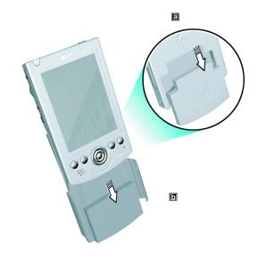
4 Slide the battery release switch on the handheld to Lock position.
