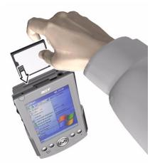
3 Push the card into the slot using your finger until you feel the card lock.
