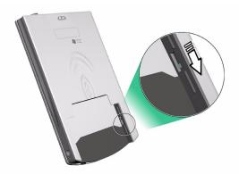
4 Insert the battery pack into the battery bay (**a**), then slide the battery release switch to the Lock position (**b**).
