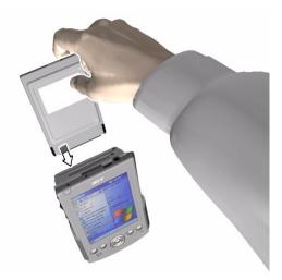
3 Push the card into the slot using your finger until you feel the card lock.
