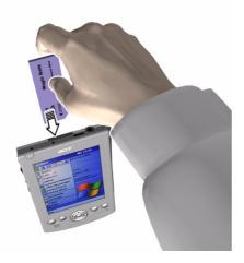
3 Push the card into the slot using your finger until you feel the card lock and hear an audible system sound; this will signal that the card is already properly seated within the slot.
