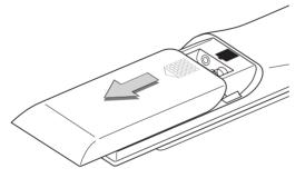
2 Insert two AAA batteries (supplied) to match the polarity indicated inside the battery compartment.
