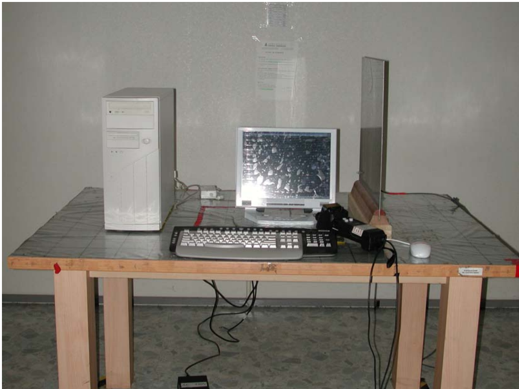
ESD Test Setup (Mode 2)
