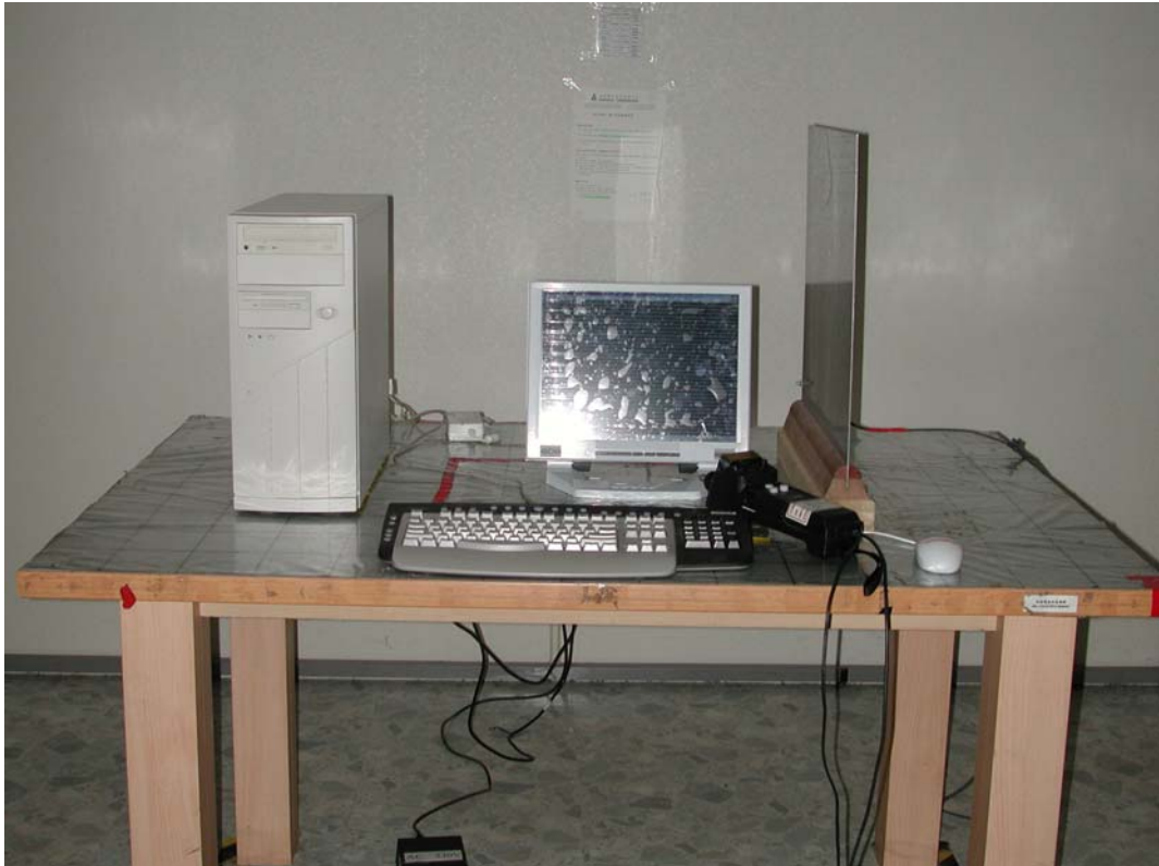
ESD Test Setup (Mode 2)
