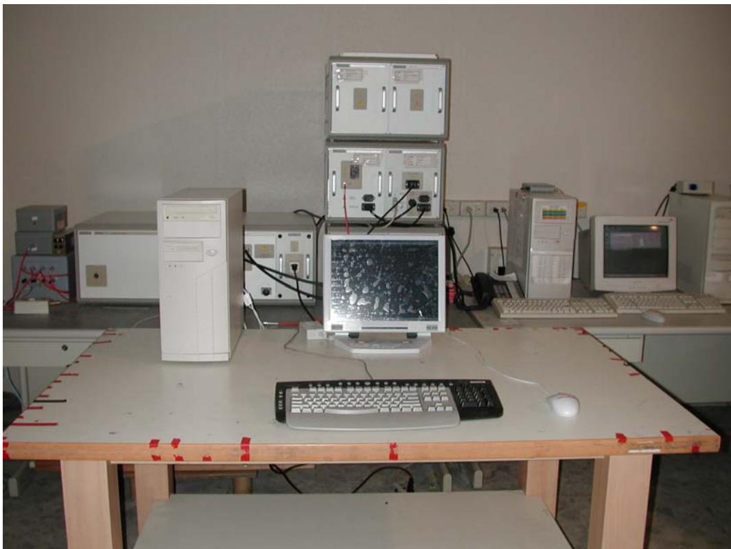
SURGE Test Setup (Mode2)
