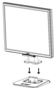
Figure 1 Installing and Removing the Swivel Base
