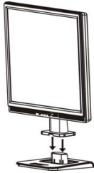
Figure 1 Installing and Removing the Swivel Base
