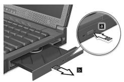
When the power is off, you can eject the drive tray using the emergency eject hole. See page 46.
