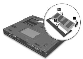
**4** Replace the memory cover and secure it with the screw.
