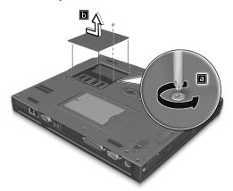
3 Insert the memory module diagonally into the slot (a), then gently press it down until it clicks into place (b).
