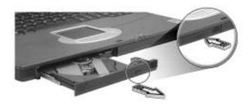
When the power is off, you can eject the drive tray using the emergency eject hole. See page 50.
