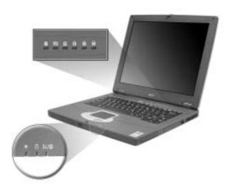
The Power and Battery status indicators are visible even when the display is closed.
