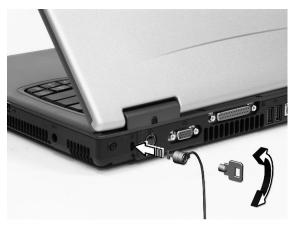
Wrap the computer security lock cable around an immovable object such as a table or locked drawer handle. Insert the lock into the notch and turn the key to secure the lock. Some keyless locks are also available.
