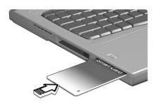
To remove the SmartCard press the SmartCard (a) and remove the SmartCard (b) as shown in the illustration below.
