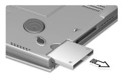
4 Insert a new hard disk module into the hard disk bay and tighten the hard disk bay screw.
