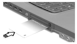
To remove the Smart Card first press the Smart Card (a) and remove the Smart Card (b) as shown in the illustration below.
