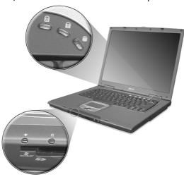
The Power and Battery status indicators are visible even when the display is closed.
