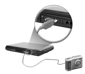
USB is plug and play, which means that you can connect and start using a USB device without having to restart your computer. You can also disconnect the device at any time.
