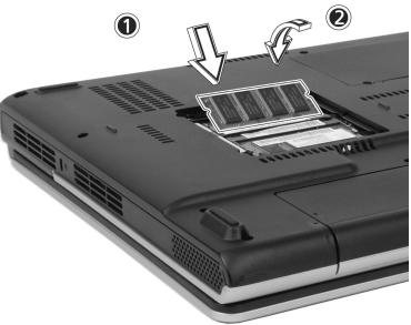
4 Replace the memory compartment door, and fasten the screw.
