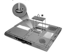
3 Insert the memory module diagonally into the slot (a), then gently press it down (b) until it clicks into place.
