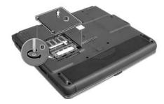
3 Insert the memory module diagonally in the slot (1), and then press down gently until it clicks in place (2).
