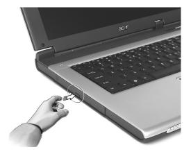
When the power is off, you can eject the drive tray using the emergency eject hole.
