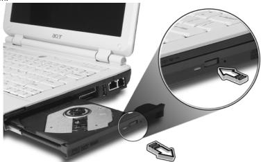
Insert a paper clip to the emergency eject hole to eject the optical drive tray when the computer is off.
