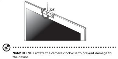
For your convenience, the camera snaps to 45 degrees to match the position of your face in front or at the back of the LCD panel.
