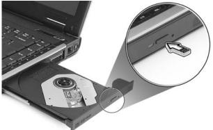
Insert a paper clip to the emergency eject hole to eject the optical drive tray when the computer is off.
