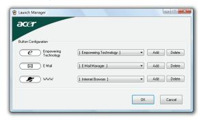
Launch Manager allows you to set the four easy-launch buttons located above the keyboard. **"Easy-launch buttons" on page 27** for the location of the easy-launch buttons.
