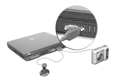
USB is plug and play, which means that you can connect and start using a USB device without having to restart your computer. You can also disconnect the device at any time.
