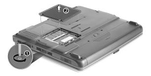
3 Insert the memory module diagonally in the slot (1), and then press down gently until it clicks in place (2).
