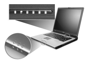
The Power and Battery status indicators are visible even when the display is closed.
