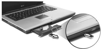
When the power is off, you can eject the drive tray using the emergency eject hole. See page 54.
